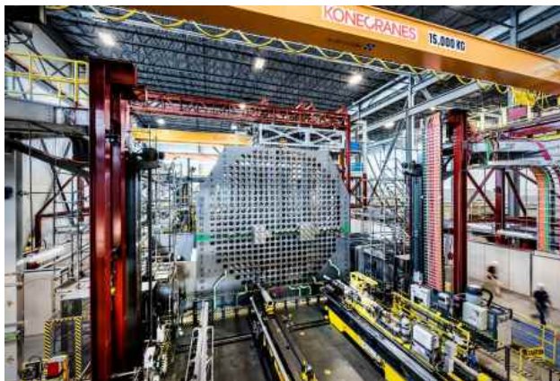
OPG's mock-up reactor is used to test tools and procedures and to train staff (Image: OPG)
