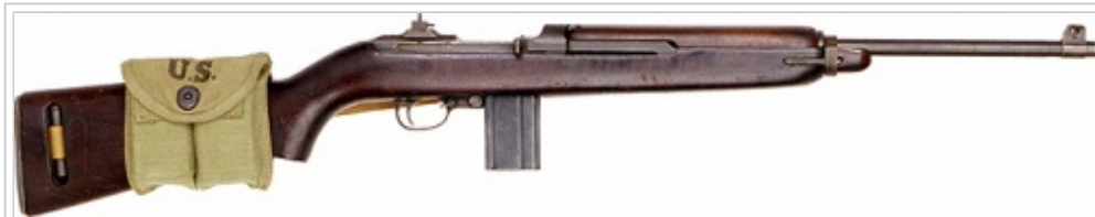
World War Two Era M1 Carbine, with Dark Walnut Stock, 'L' peep sight and no bayonet lug - correct for most of WWII, shown with khaki sling and oiler and a period Magazine pouch for buttstock
