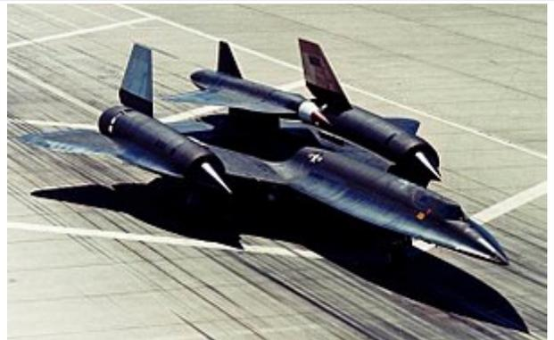
The D-21 mounted on the back of the M-21. Note the intake cover on the drone, which was used on early flights.
