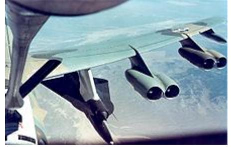
A modified D-21 carried on the wing of a B-52
