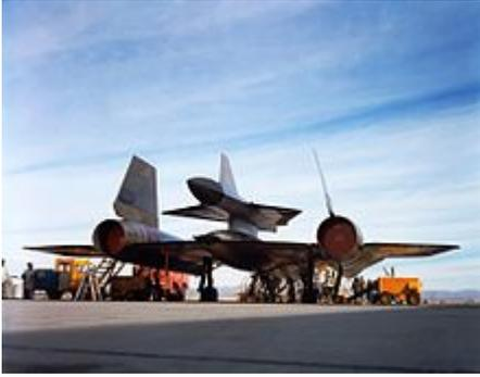
Rear view of the D-21 and M-21 combination on the ground, showing the exhaust shroud used on early flights
